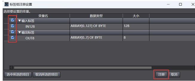
Fig92. PLC EIP-Registration setting interface
