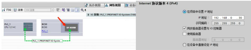
Fig73. PLC Profinet-Set the IP address of the reader for the P rofinet connection with the PLC
