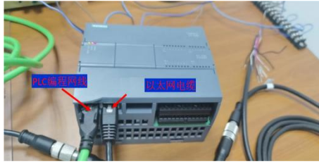
Fig68. Schematic diagram of the PLC wiring
